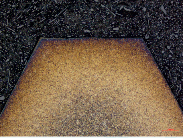
Etched with 3% Nital, BF, 50x
